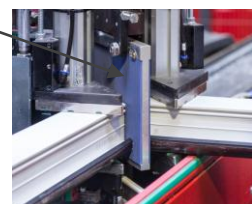
Our new, unique serrated weld plate Resulting in a stronger "zip" weld
